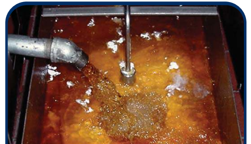
ALLOW OIL TO RECIRCULATE FOR 5-7 MINUTES
