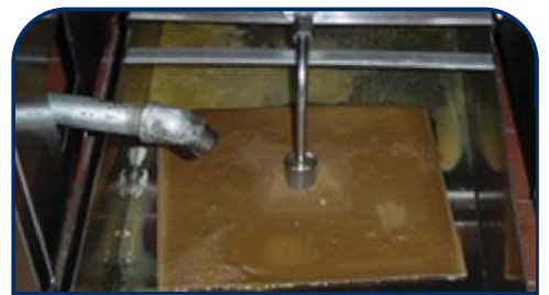
DISCARD FILTER PAPER & THE MAGNESOL RESIDUE. CLEAN YOUR FILTER PAN TO ENSURE THAT IS READY FOR USE.
